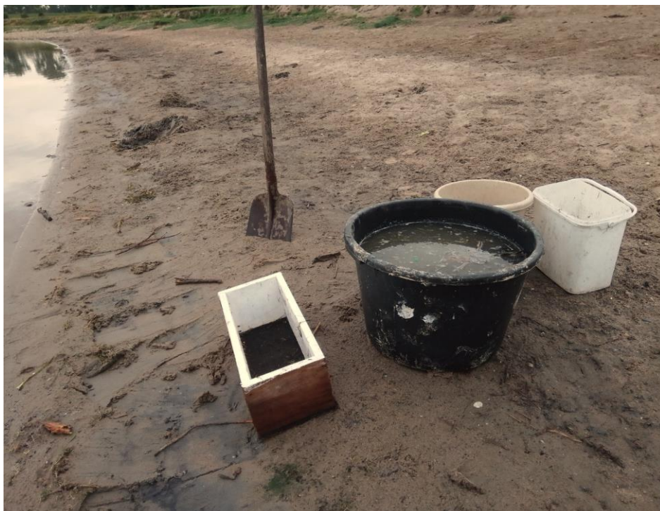
Image: The 'washing installation' consists of a pan shovel, mortar tub, and fine-mesh sieve.
